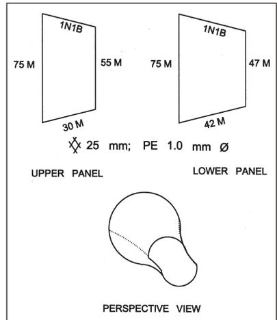
**Figure 6d.** Construction of the accelerator funnel.
