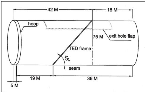
**Figure 6c.** Fixing the grid at the correct angle.
