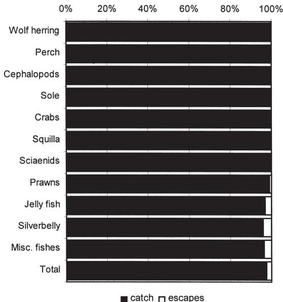
**Figure 5.** Relative exclusion rates of different species groups due to installation of CIFT-TED, during experimental trawling off Kochi.
