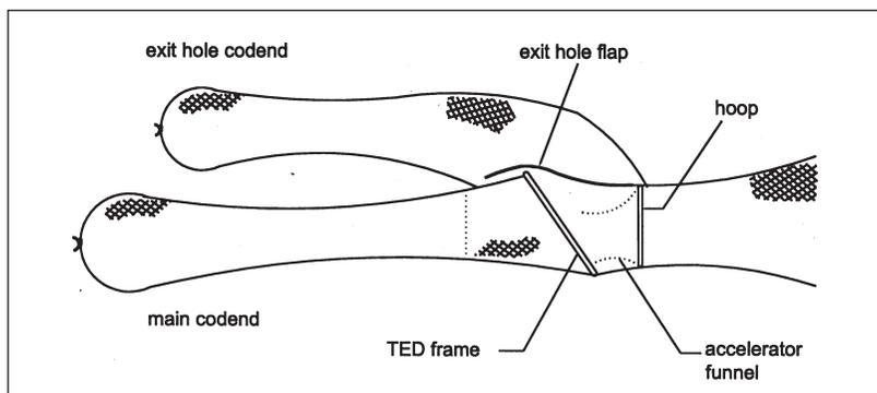
**Figure 3.** Details of rigging of exit hole codend for experimental operations.
