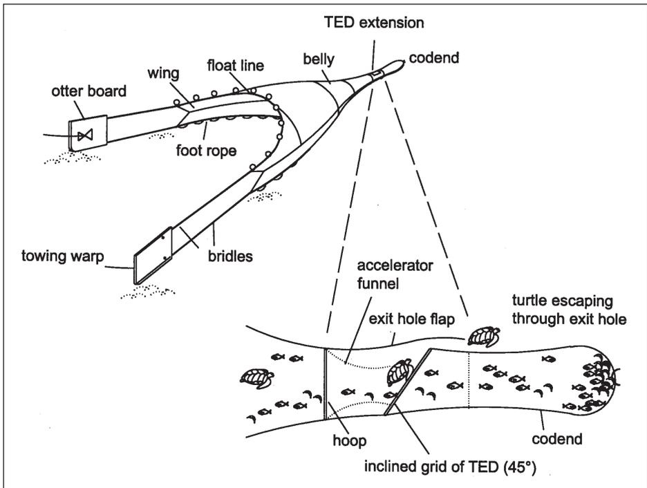
**Figure 1.** Principle of TED operation.
