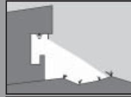
**Better:** Completely shielding fixtures with a sheet of metal flashing can reduce stray light reaching the beach.
