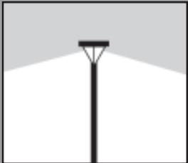
**Pole-Top-Mounted Cutoff lighting, "Shoebox" fixture.**
